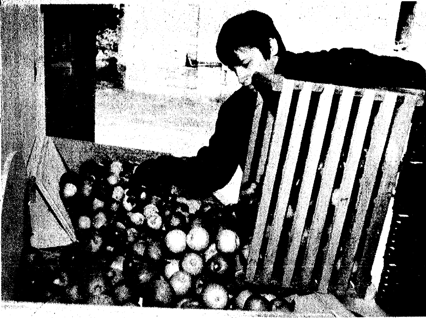
MARILYN BEGRES, of Lakeview Farms, loads a mixture of Paula Reds, Early Blaze and McIntosh apples into a bin in a drive-through between the new cider press room and a 1,000-bushel capacity, 36 degree apple cold storage room. The bin has an attached conveyor belt which moves the apples into the washer through the opening to the lower left.
