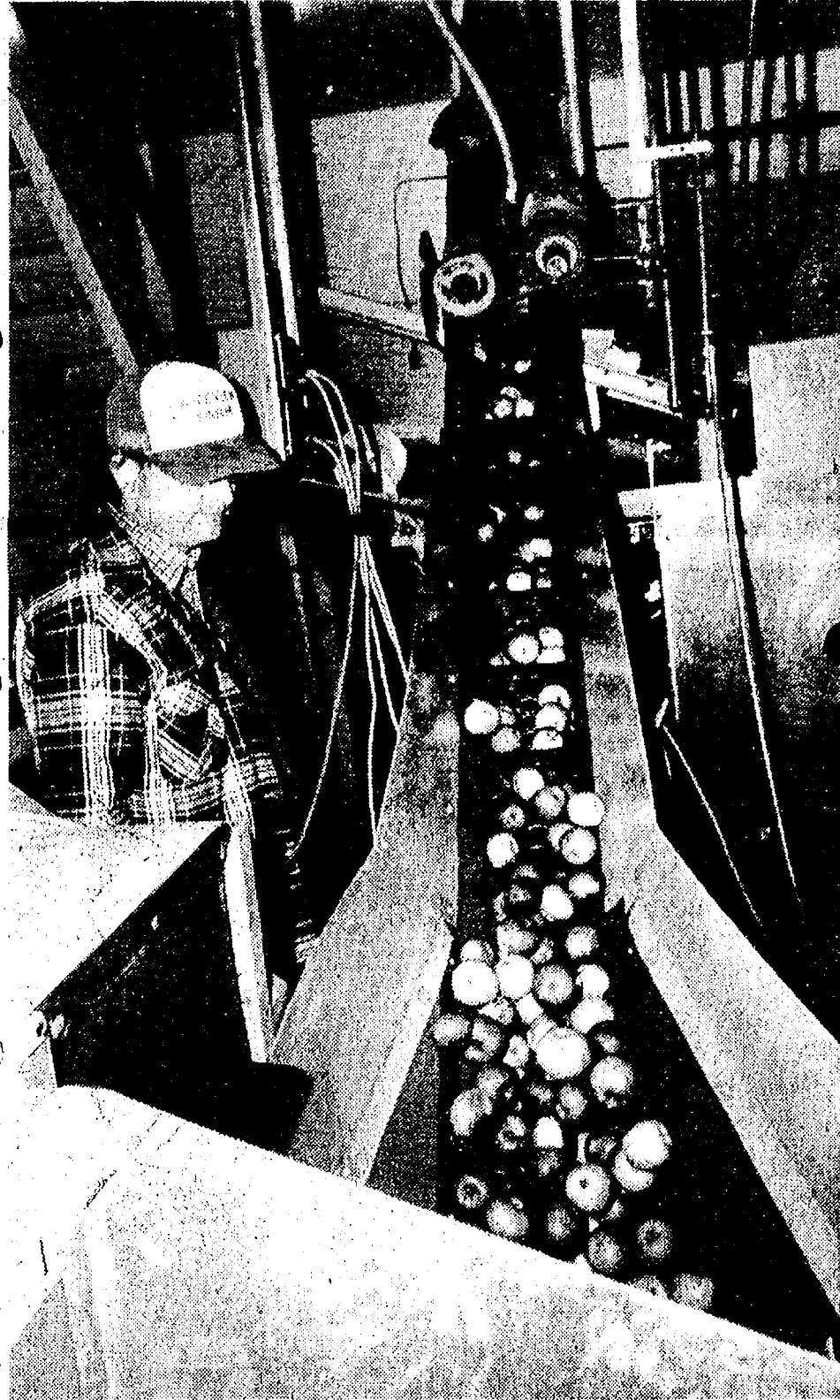
THE APPLES, washed and brushed dry in the box-like machine to the left, move up this paddle conveyor and fall with a thunk into the folding cloths below. The controls for the different motors are conveniently placed, beside Woody Begres' head.
